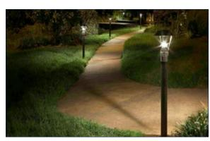
Bollard lighting that minimizes the light directed outside of the trail corridor.
